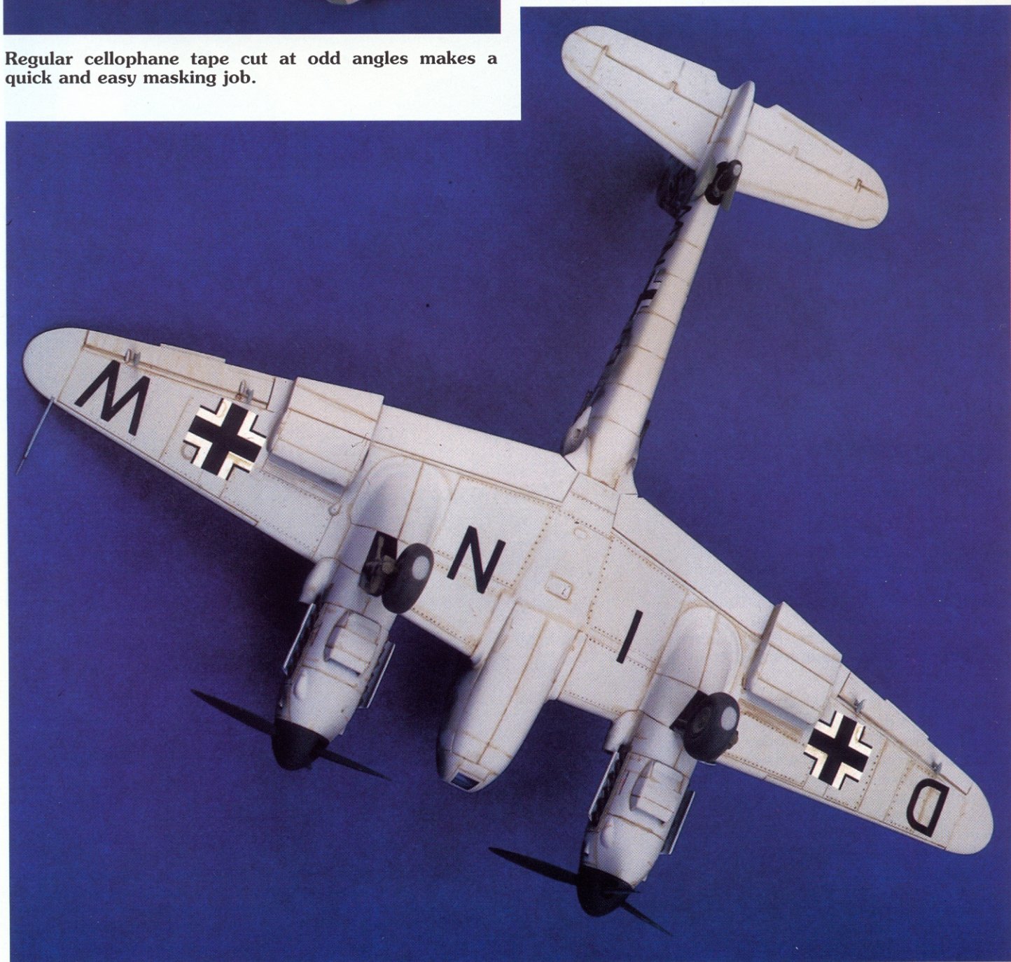
Light washes were applied to the light and lower surfaces. The tires have been slightly flattened by rubbing the completed model on a large sheet of fine grit sandpaper.
